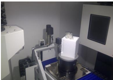
Fig. 1. Measurement element inside the chamber of CT scanner METROTOM 800
