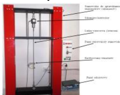
Fig. 4. Strain gauges testing set in 2MCL
